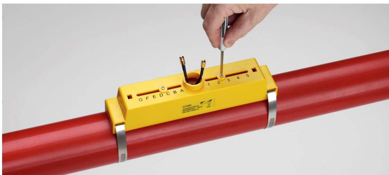
Figure 20 Removing sensor-holding screws
