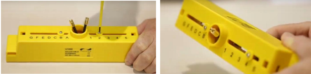
Figure 14 Loosen the flow sensor-holding screws (left); slide to correct position (right)
